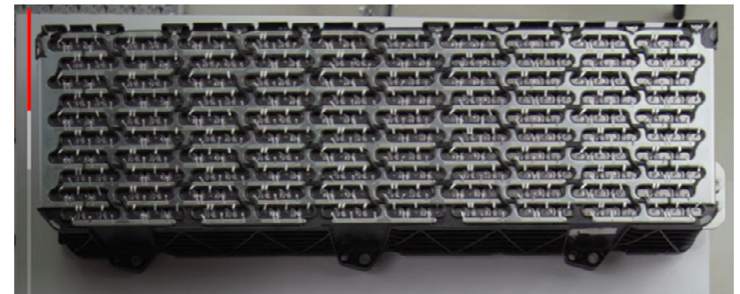
LuCid Air modul housing & contactor plate moulded by Plastikon Industries
