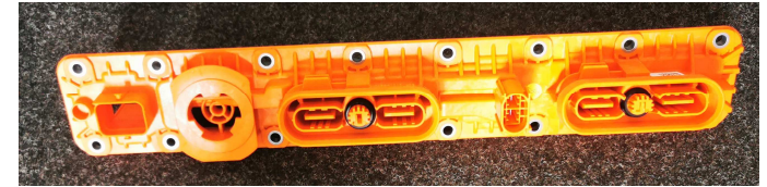
HV Battery MEB-Plattform Volkswagen – connector plate
